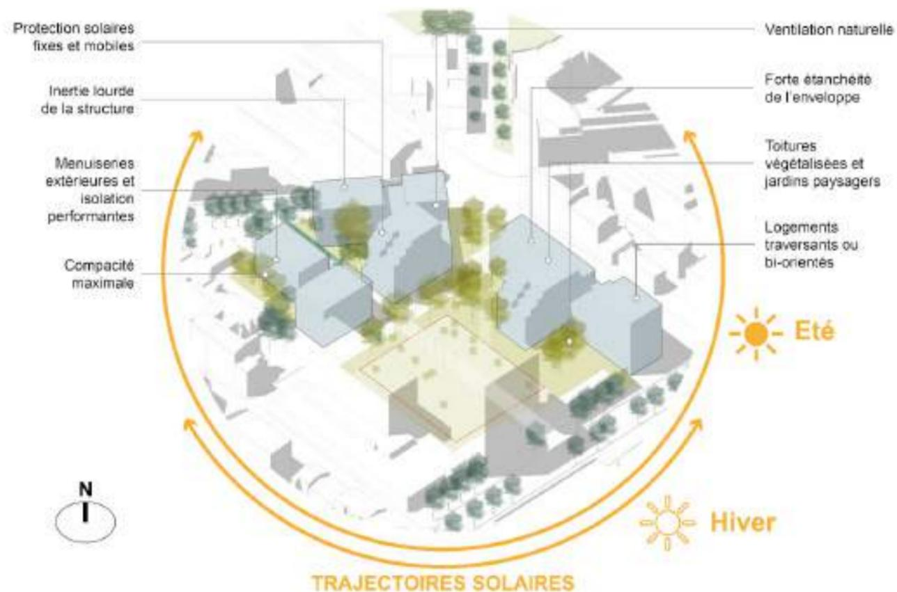
FIGURE 2 : PRINCIPALES CARACTÉRISTIQUES DE LA CONCEPTION BIOCLIMATIQUE
